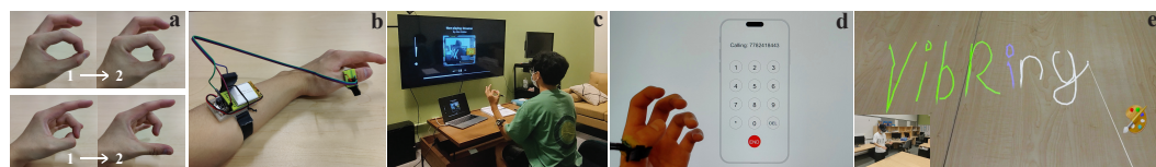
Fig. 1. (a) Example uncommon gestures included in our gesture design set. Top: Gesture “PN_rub”, where the index fingernail rubs (scratches) the thumb’s pad; bottom: “NP_flick”, where the thumbnail presses on the middle finger’s pad and flicks away. (b) VibRing’s wearable platform including an armband encasing the ESP32 Adafruit Feather chip and a thumb ring consisting of a DC bias circuit and a conditioned piezoelectric disk. Demonstrated online applications including (c) a music player, (d) a phone dialer, and (e) an AR painter.
