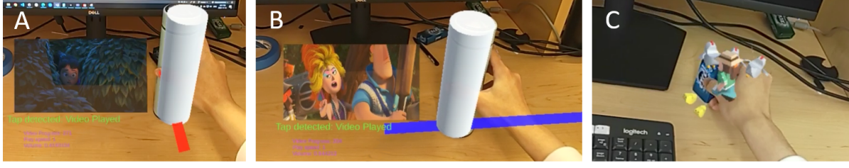
Figure 7: A demonstration of the user study setups: (A) a y-directional translation movement of the controller object adjusts the volume of the video player. A vertical virtual bar is rendered to indicate the control range. (B) an x-directional movement controls the play head. A horizontal bar indicates the progress bar. (C) The AR game: Farm, where the tangible object is used as a physical proxy of the game character.
