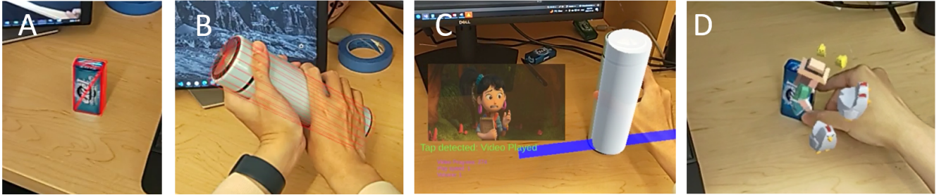
Figure 1: TangiAR enables tangible interactions using everyday objects in immersive augmented reality. (A) TangiAR tracks the 3D position and rotation of objects without the need for additional visual markers or texture registration, (B) even under substantial occlusion. We showcase the performance of the system with two example applications: (C) a tangible controller for an AR video player; and (D) an AR game: Farm, where the object is used as a tangible proxy.
