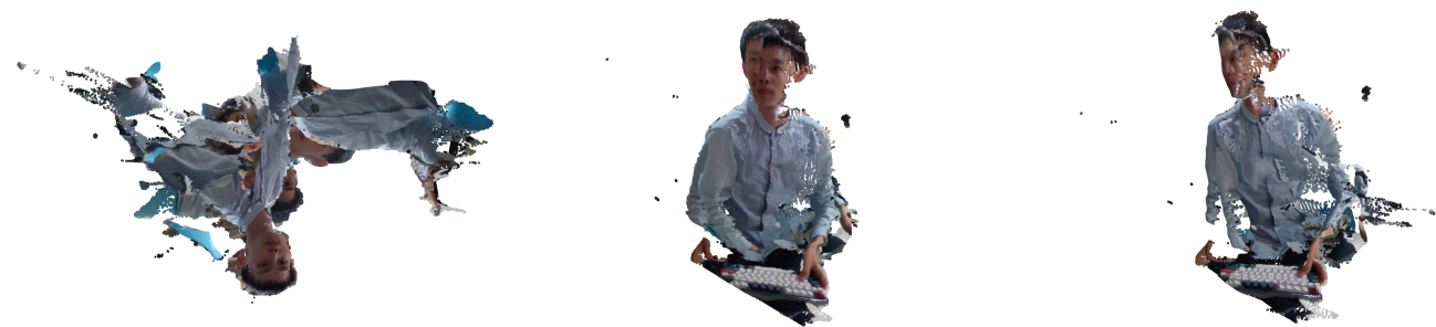
Fig. 10: Registration results for test user 1 sitting sideways using All Points+PFHRGB+point-to-point. Left: initial point clouds; Middle: after coarse registration; Right: after ICP registration.
