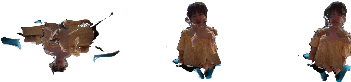
Fig. 8: Registration results for test user 2 sitting up straight using All Points+FPFH+point-to-point. Left: initial point clouds; Middle: after coarse registration; Right: after ICP registration.
