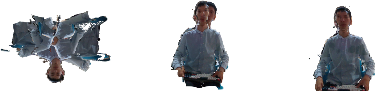
Fig. 7: Registration results for test user 1 sitting up straight using All Points+FPFH+color-ICP. Left: initial point clouds; Middle: after coarse registration; Right: after ICP registration.
